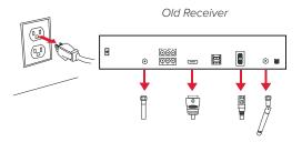
**Set Up Your New Receiver.** Attach the cables and remote antenna to your new receiver. Then, plug the new power cord into the wall.
